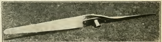
© U. S. Army Air Service Fig. 5—Reed propeller with boisted flange hub
